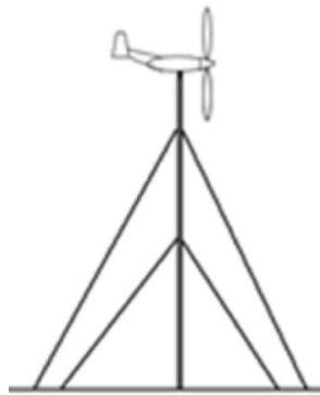
Figure [10]: Guyed Mast
